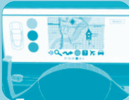
City driving display. Note, from left to right, the collision avoidance system view (the car image), the global positioning map with an arrow showing the car's location, and the speed. The three colored dots—red, yellow, and green—are there to warn the driver about road conditions or traffic. If conditions change, one of them will blink and thereby warn the driver to pay closer attention.
