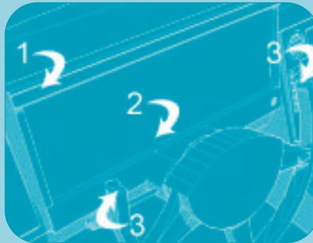
The display screen with the steering wheel. 1. Upper interface. 2. Main screen. 3. The switches on the steering wheel.
