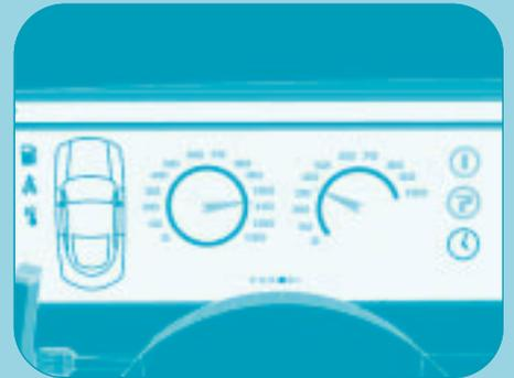
Highway driving display. From left to right, Gas, seat belt, and temperature icons; collision avoidance system view; speed; and RPM.
